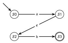
Now, I would say that we are done at this point, as we have a machine that accepts only the concatenated string, with one starting state and one final state (having only one final state is not a restriction of a FSM, but having only one allows us to inductively build our machines here). If we really wanted to, we could optimize the machine a little bit, but it is not necessary.
