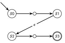
To take our previous example of  $R_1$  being /a/ and  $R_2$  being /b/, when we want to concatenate these machines we get the following machine:
