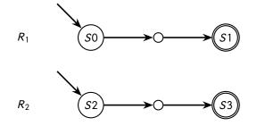
Now we don't know what regular expression  $R_1$  and  $R_2$  are, just that they have 1 starting state, and 1 accepting state. The small, unlabeled nodes here just represent any internal nodes could exist (if any).
