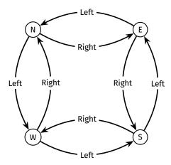
This graph represents a finite state machine. A physical machine can be made to do these things, but for the most part, we will emulate this machine digitally. We typically define a FSM as a 5-tuple:
